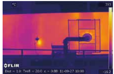
These images form part of a weekly inspection done. The images are analysed to detect refractory degradation or product build-up on the inside.
