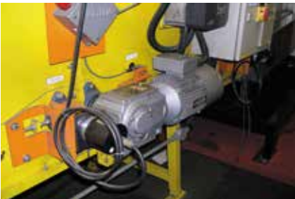
Visual and thermal image of a motor and a gearbox at Heathrow's baggage handling system.
