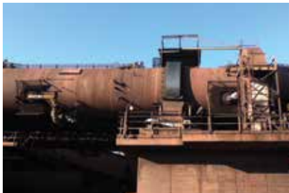
These images form part of a weekly inspection done. The images are analysed to detect refractory degradation or product build-up on the inside.
